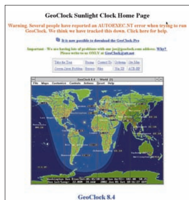
Fig. 1: Geoclock showing the grey-line terminator that has enhanced propagation.
