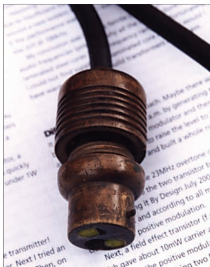
Fig. 1: The bayonet bulb adapter socket was once very popular- Phil G4JCP says that this wooden version still works! (see text).
