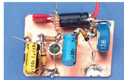
Fig. 2: The circuit lends itself to 'Ugly' construction (see text).
