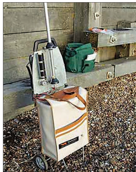
The shopping trolley Amateur Radio station used by Andy Foad G0FTD.
