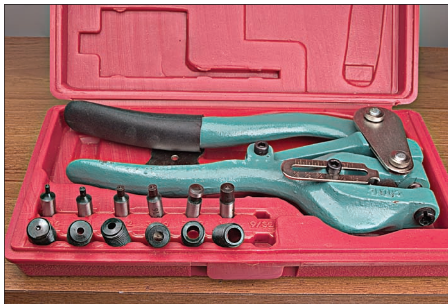
Fig. 1: The hand-punch obtained by Rob G3XFD - with the help of George G3RJV. It enables the operator to punch small discs of p.c.b. material to make 'copper islands'. These are then fixed to the p.c.b. using Cyanocrylate adhesive (see text).
