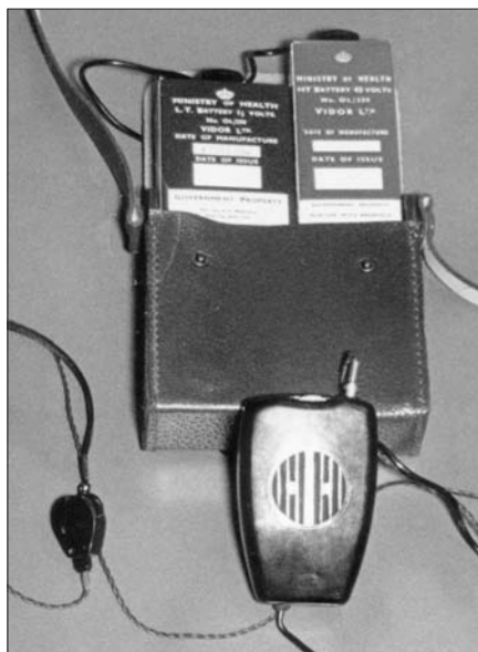
Fig. 2: The Mesdresco miniature valved hearing aid was the first to be available from the National Health Service in 1948. For its time the hearing aid was a marvel of miniaturisation- although the batteries had to be carried in a separate pouch! Photograph courtesy of the Royal National Institute for the Deaf.
