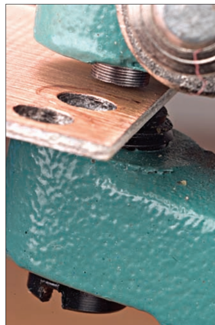
Fig. 3: Close - up view of the hand punch in use making one island. Two previous holes may be seen. Note the end of the die visible under the punch lower jaw.
